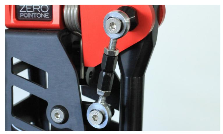
6 – Adjust the Shifter to ensure all gears are properly engaging. This is achieved by adjusting the turnbuckle that moves the 'swingarm' which in turn centralises the gear stick. Loosen both M6 nuts to turn the black turnbuckle and ensure they're fully tight once finished.
