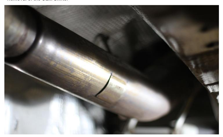
1 – The first step is to gain access to the OEM shifter by removing the exhaust and heatshield. The full system does not need to be removed, but the exhaust does need to be dropped allow enough clearance to the shifter area. The exhaust tunnel heatshield will need to be fully removed to access the shifter.
