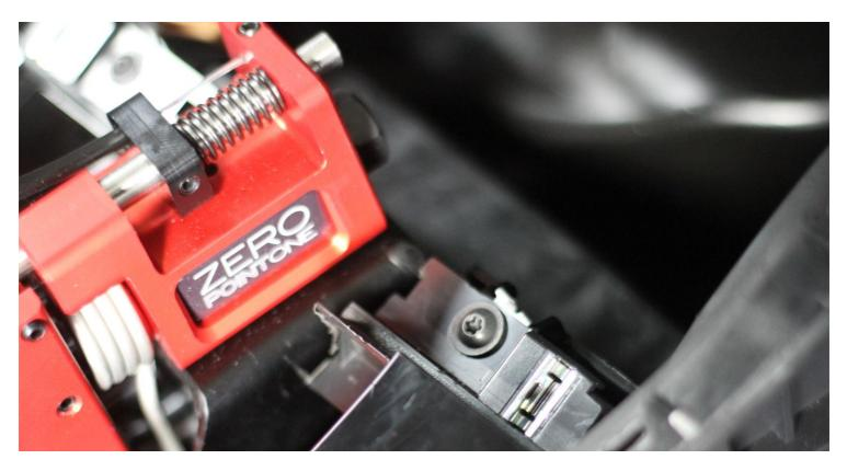
7 – Once the ZeroPointOne Shifter, the centre console is ready to go back on, but will require trimming. This will be in a different position for each vehicle that the ZPO VW/Audi/Seat/Skoda Shifter fits and we will be making templates for each model that we can get information for. A Dremel or grinder will make light work of cutting the plastic and leave a clean cut.
