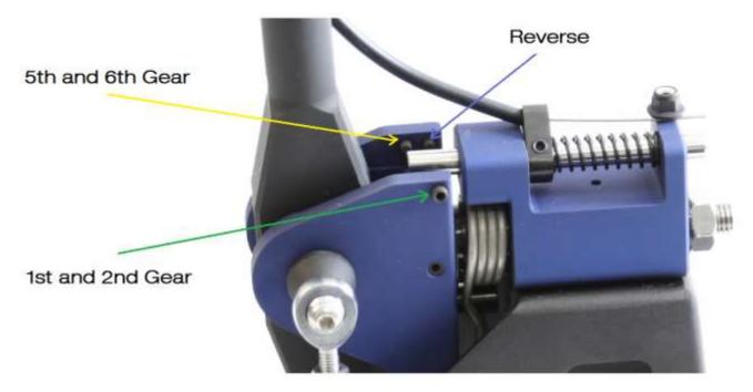
Using the gear lever, shift the gearbox into 1st and 2nd. You may need to screw the (green arrow) grub screw out to achieve this.
