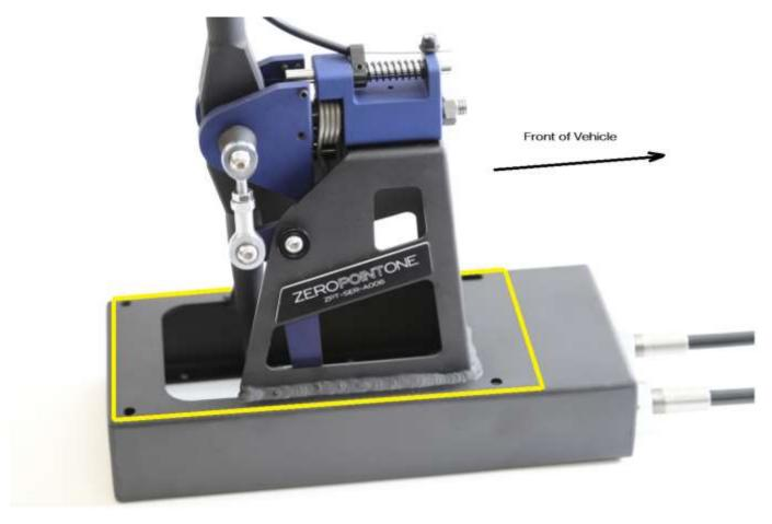
The yellow line shown on the base of the ZPO shifter is a guideline of where the foam/sealant should be placed.
