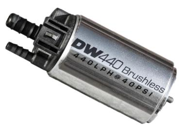
The DW440 brings brushless pump technology INTO the fuel tank. With a total height of only 4 inches (102mm), it is the only highflow aftermarket brushless pump that is easily retro-fitted into an OE pump module. Brushless technology reduces friction and heat, increases effeciency, vastly improves pump lifespan in ethanol and methanol fuels, and allows higher voltage inputs for increased flow.
