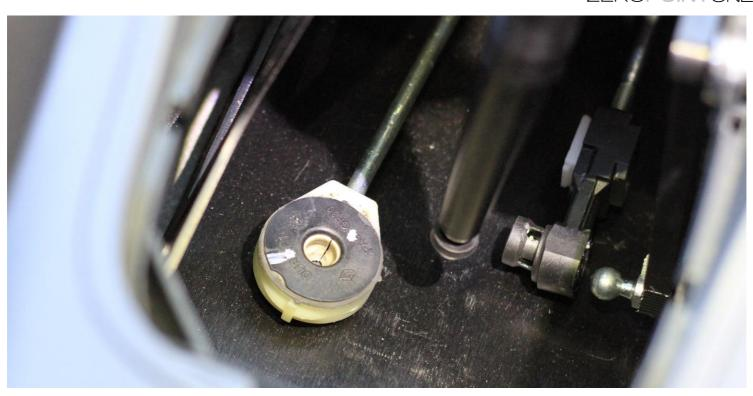
18 – Once the shifter has been seated correctly on the four M8 studs and the cables have been located into their correct positions on the shifter base, the cable ends can be connected to the shifter ball studs. Once both are connected, push the white plastic fixing into position on the threaded rod, securing the cable into position.
