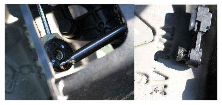
12 – Remove both cable ends from the shifter ball studs. The gear stick cable can be removed by twisting it off the ball stud. The swing arm cable is removed by pulling out a black cup that locks onto the ball stud, a small flat headed screwdriver can be used to help the cup out of its closed position.
