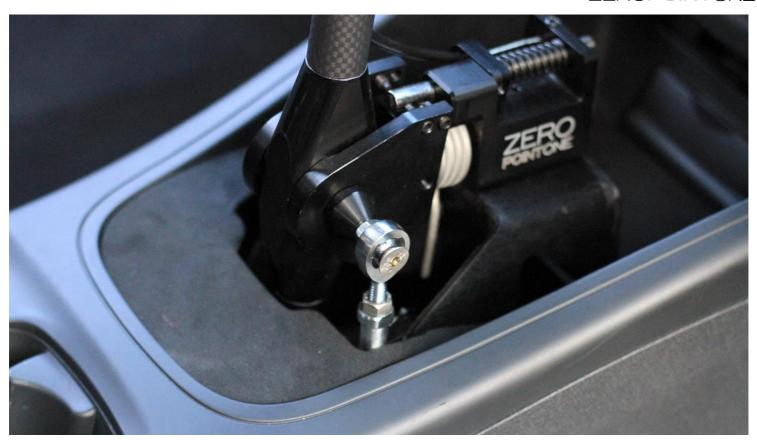
22 – Install the centre console cover plate provided, ensure this is seated correctly to avoid rubbing on any of the components.
