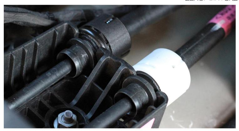
11– Pull the white and black sleeves back on the OEM shifter cables to release them from the shifter base. This will then allow you to lift the shifter off of its mounting studs and twist it on its side to access to the cable ends.
