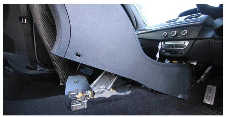
6 – Now that centre console is free to move, it can be raised enough for you to begin unclipping the various wired in electrical items. The 12V point at the rear of the console, the cruise control/speed limiter button in the middle, nav/display controller if the option is fitted and then the audio connections at the front.
