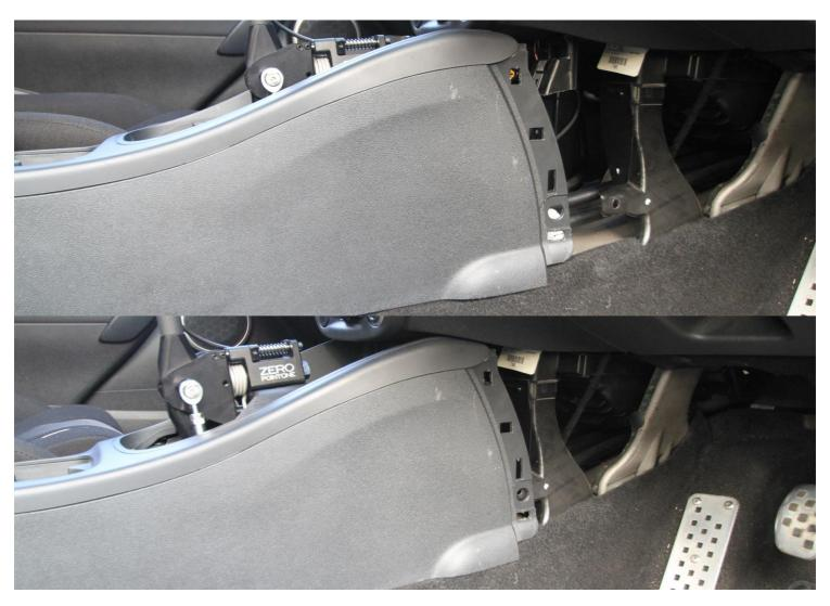
20 – Move the console towards the rear of the vehicle in order to tighten the two rear nuts on the shifter, then forward to tighten the front two nuts on the shifter.
