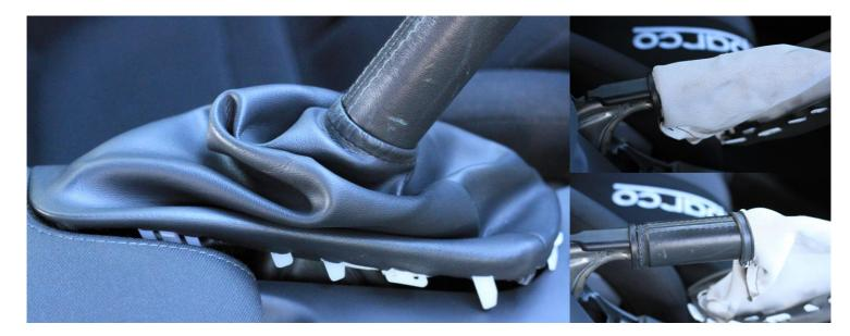
4 – Unclip the handbrake gaiter in the same manner as the gear stick gaiter surround. Use interior trim tools to avoid marking the console. Once unclipped, the handbrake gaiter can be pulled up and over the leather handle.
