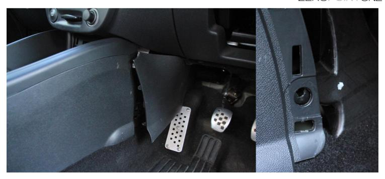
5 – Remove the trim connecting the centre console to the instrument panel (dash), there are three metal clips that can be prized out of their mating holes with a plastic interior trim lever bar. Once the plastic trim is removed, a fir tree fastener needs to be removed from the hole shown in the picture.
