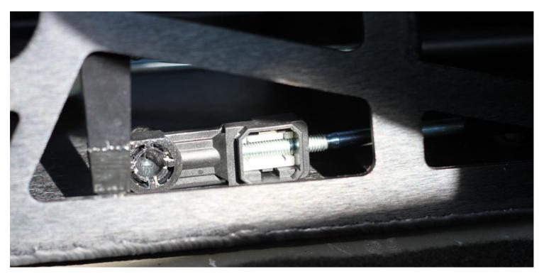
16 – Before putting the centre console in the vehicle, be sure to push the white plastic fixing out and away from the thread that it is holding in place. This will allow the cable end to move and eventually clip onto the ZPO shifter swingarm ball stud without pulling the cable away from its neutral position.
