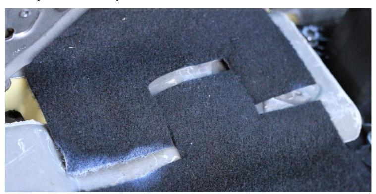
8 – Cut a slit in the carpet that covers the foam NVH material underneath the handbrake, this will give you access to an airbag module cover that needs removing. The above picture shows an overly complicated method of cutting the carpet, which would allow a single piece of tape to secure it back together, but a single straight cut would be just as effective.
