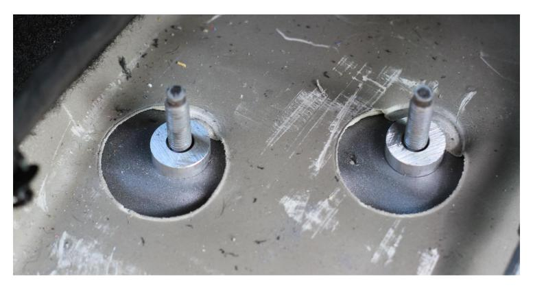
14 – Place the supplied spacers over the M8 studs, these will allow the shifter to sit on a hard surface rather than the foam NVH material, resulting in a better residual torque over the lifetime of the shifter.
