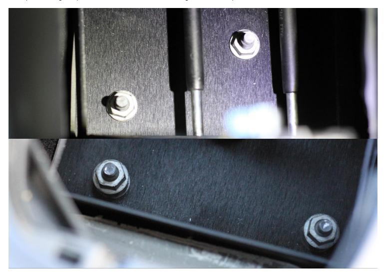
19 – The four nuts can now be tightened. 25Nm is sufficient for this joint, any more than this and you will strip the thread of the weld stud and damage the shifter base.
