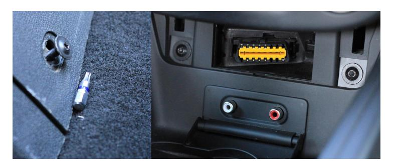
2 – Remove the four tapping screws that secure the centre console to the car. There are two screws at the front of the console underneath a plastic trim where it connects to the instrument panel,. The other two are either side of the centre console, in the rear lower quarter and will require the seat to be moved forward to gain access. These require a T20 Torx bit to remove.
