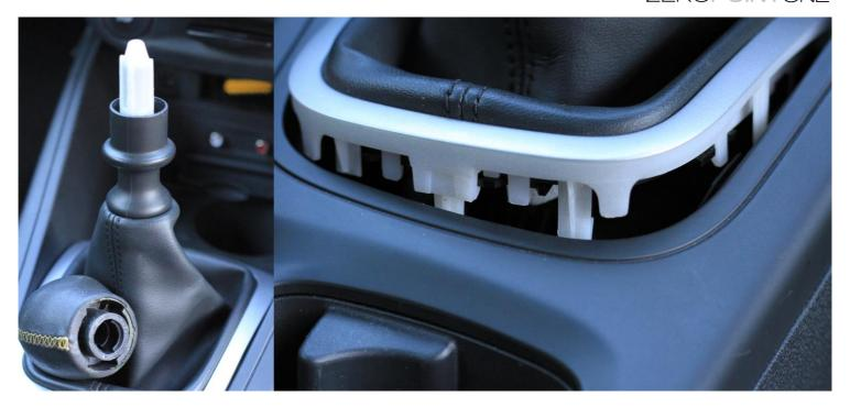
3 – Pull the OEM gear knob upwards to release it from the shifter, then unclip the gaiter surround from the centre console using interior trim removal tools to prevent damage. Once removed, you'll be able to pull the entire gaiter and surround up and off the shifter stick
