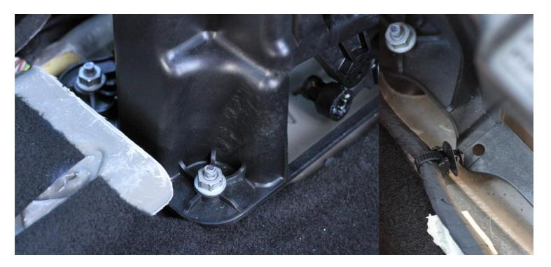
10 – A 13mm socket is required to remove the four M8 nuts that fasten the original shifter to the vehicle body. Once removed, these need to be kept safe so that they can be used for the ZPO shifter installation. Release the centre console wiring attached to the shifter by removing the two fir tree clips that are cable tied to the wiring bundle.
