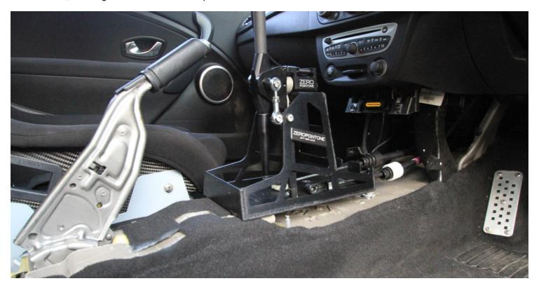
15 – The ZPO unit can now be placed in the vehicle. If you are fitting the centre console back in, then do not put the shifter over the weld studs, instead, rest it on top of them. This will allow you to move it backwards and forwards when re-fitting the console. The cables will need to go into position, but not yet connected to the base or the ball studs.
