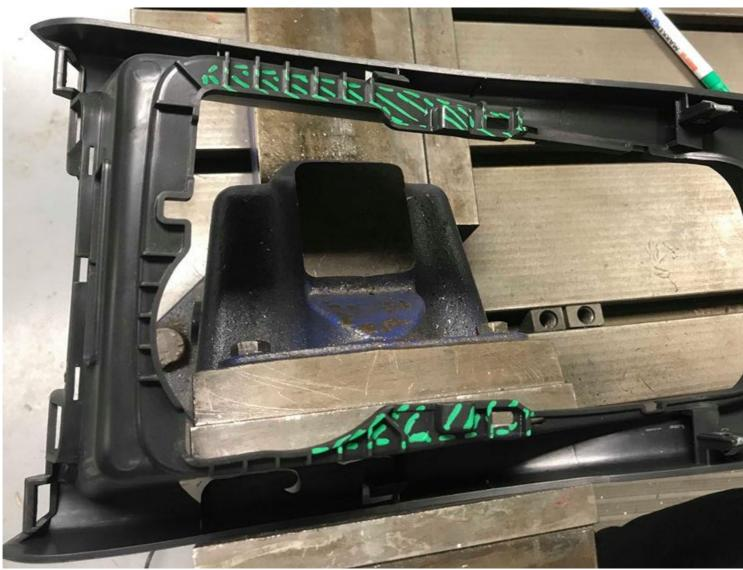
13 – A small section of the centre console top section needs to be modified before fitting it back in the vehicle. This is easily done with a Dremel or similar device. The areas marked with green pen in the above pictures give an indication of where you should trim.
