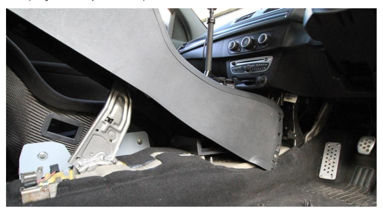
17 – The centre console can now be placed over the shifter and handbrake. (Tip, pull the handbrake up as high as possible to make this job easier). Ensure you have the newly modified top section of the centre console in place before fitting, it cannot be installed after the centre console has been installed. Reconnect all wiring.
