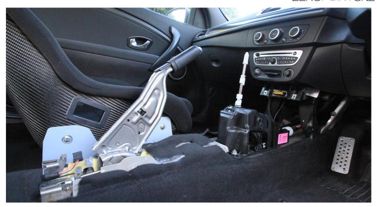
7 – The centre console can now be removed and taken out of the car. A foam surround needs to be taken off the original shifter to gain access to the mounting nuts.
