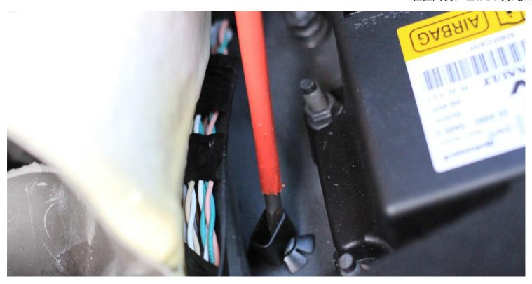
9 – The airbag module cover is secured into position with a plastic nut that can be removed with a flat head screwdriver. Fold back the foam NVH material and push back the wiring that covers the back end of the airbag module cover. The plastic nut can then be accessed and removed, releasing the cover and allowing access to the retaining M8 nuts on the original shifter. The above picture does not show the cover, but illustrates where you will find the nut relative to the airbag module.
