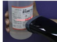
With AR-3100 series scanners, barcodes can be read from contact which greatly increases efficiency.
