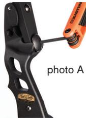
**⚠️WARNING:** Never loosen your limb weight adjustment bolts (Tiller Bolts) more than 4 turns from the bottomed-out position as it could cause the bow to violently disassemble
